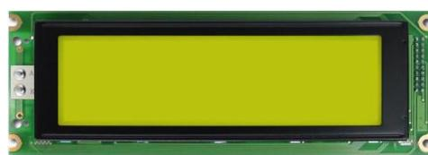
**Figura 18 - *Display* Toshiba T6963C, 240x64 pixels**
