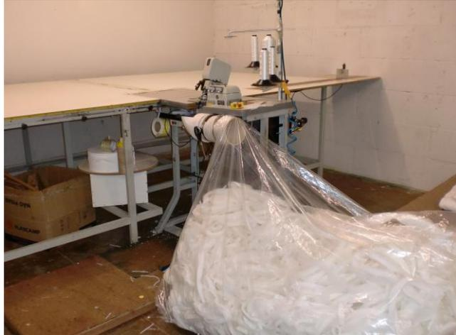
**Figura 18: Máquina de Overlock (Porter).**
