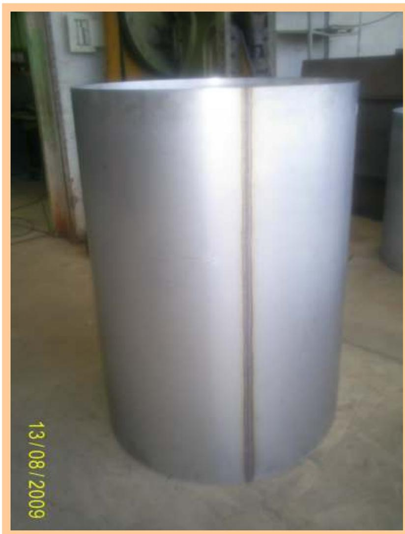
**Figura 5 – Tanque interno.**
